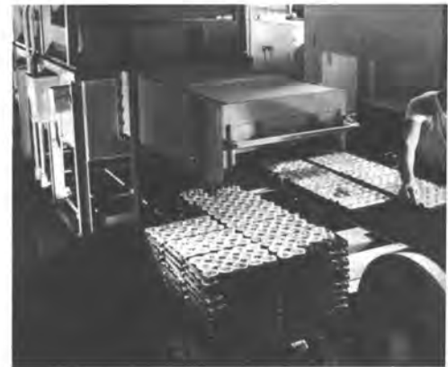
Special electric furnace for fusing the bifocal segments to the major ophthalmic lens blanks.
