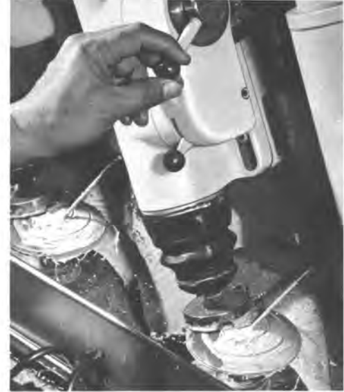
Close-up of fine-grinding of lens surface with modern diamond-impregnated surfacing tool.
