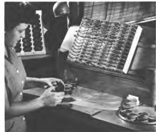
This type of equipment is used in blocking lenses, preparatory to grinding and polishing.
