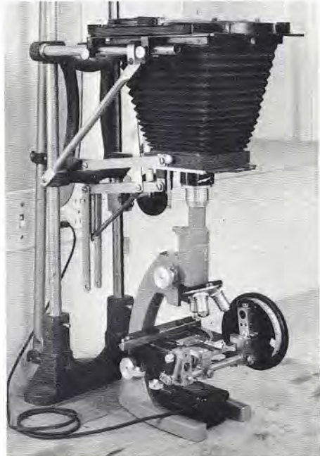
Figure 3. Microscope with micro-pressurometer attachment in position under photographic enlarger which has been converted for microphotographic use. Since this photograph was taken, a compur type shutter has been placed between the microscope tube and the enlarger bellows.
