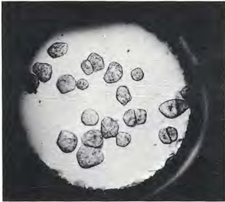
Figure 4. Pressure head with a number of individual potato cells which were reconstituted from a sample of dehydrated potato granules, 30X. By manipulation of the mechanical stage, while the pressure head remains stationary, the cells may be moved about until only a single cell remains under the pressure head for test.
