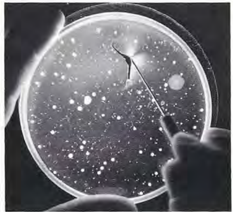
Figure 3. The area adjacent to the point of the needle appears bright due to introduction of strain birefringence in the agar as a result of the pressure of the needle.
