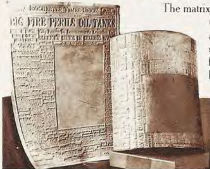
The plate at the right was cast from the cardboard mold or mat at the left
