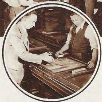
Advertisements are assembled in the ad alley, a section of which is above. Make-up of pages under direction of an editor is the last operation before stereotyping
