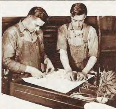
The mold, commonly called a mat, is strengthened by backing and toasting
