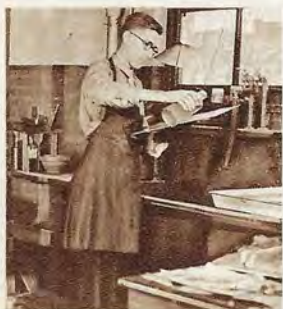
A sheet of metal is coated with a solution sensitive to light and placed in the printing frame under the halftone negative as shown at the right
