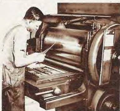
A sheet of cardboard, rolled into the type, forms a mold for the page plate
