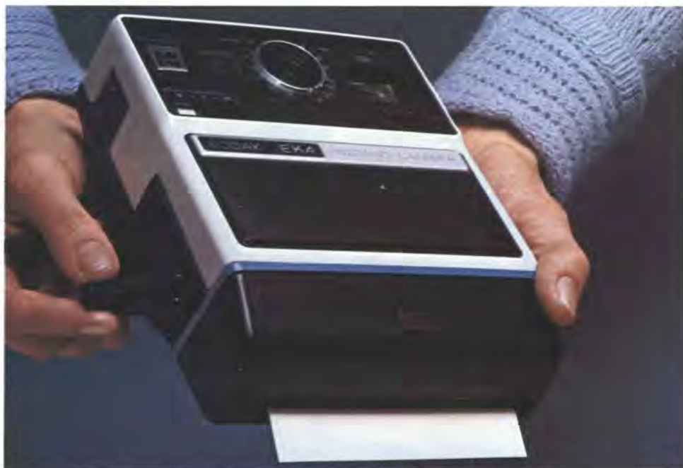
A convenient hand crank is used to eject the picture unit from the Kodak EK4 camera.
