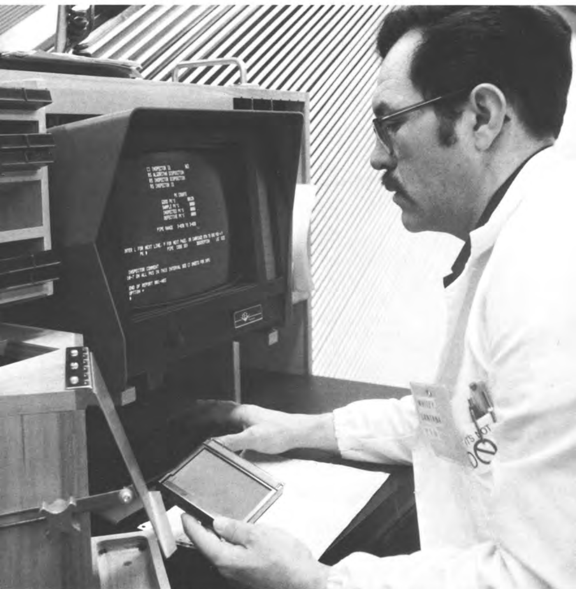
The diagonal storage racks rising behind the operator here house thousands of lighttight packs of Kodak instant print film. A computer "knows" their whereabouts and, after extensive inspection, approved packs are released for shipment. Its reports are displayed on the screen in foreground.
