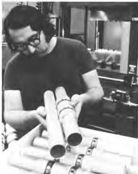
Capital expansion at Kodak Apparatus Division includes efficient manufacturing processes, such as bulge forming to mold polyurethane material to specified shapes and sizes.
