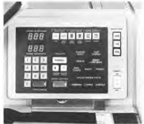
The display panel of the new line of Kodak Ektaprint copier-duplicators with positioner and sorter virtually tells the untrained user how to operate the machine.
