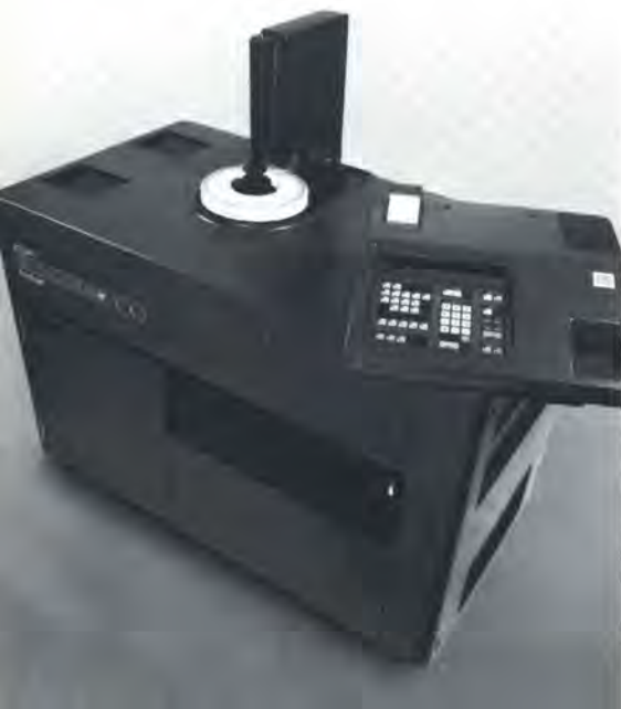
Ektachem 100 analyzer performs colorimetric testing.
