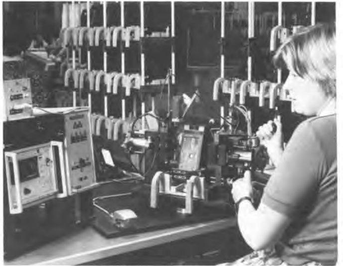
Monika Wacht tests the shutter of a Kodak EK8 instant camera.
