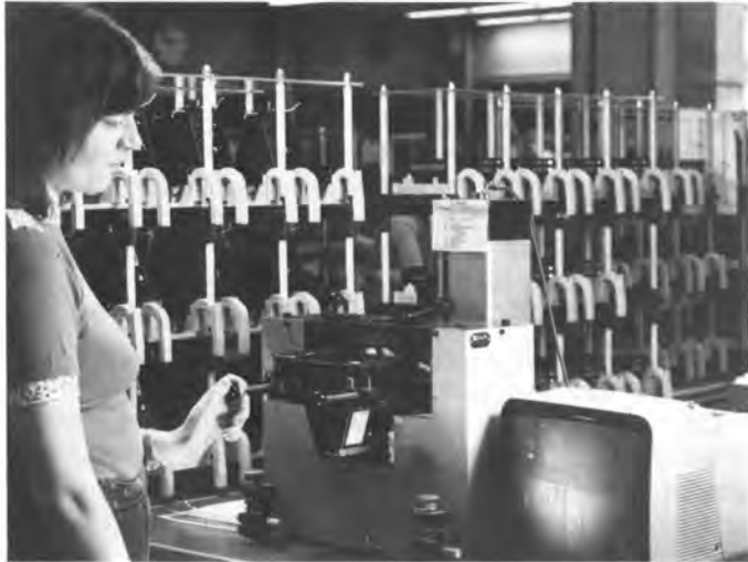
Hildegard Schulz examines the film plane of the Kodak EK8 instant camera relative to optical axes by means of a monitor display.
