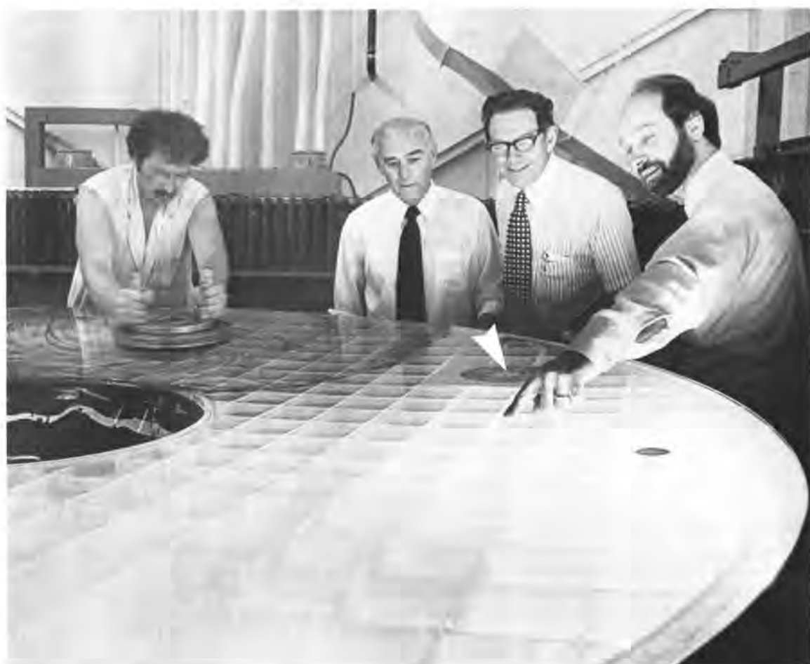
Sam Baubie, left, fine polishes the mirror blank in KAD's Special Optics Fabrication Dept. Jack O'Grady, department head; Dr. Frank Hicks, and John Spina, KAD Research and Engineering's project manager for the mirror, study the circular contour map (see arrow) of the mirror surface, noting high spots which must be polished to specification.
