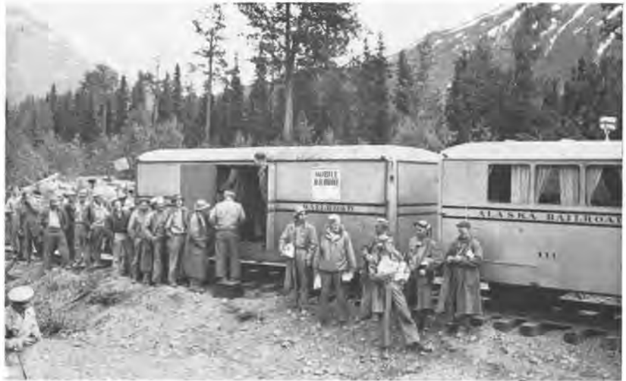
Signal Corps Photo The PX (Post Exchange) is found wherever American soldiers are stationed, but this Alaskan railway PX is unique. It is a motor truck, mounted on rails, drawing a trailer which contains the counter over which goods are sold.
