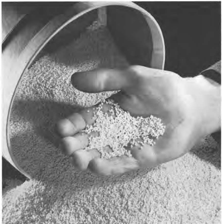
Speedy ousting of carbon is accomplished by the Army Air Forces with the aid of Tenite pellets in sandblasting equipment. The pellets are prepared for this important job by the Tennessee Eastman Corporation, do a thorough job on piston walls and piston-ring grooves
