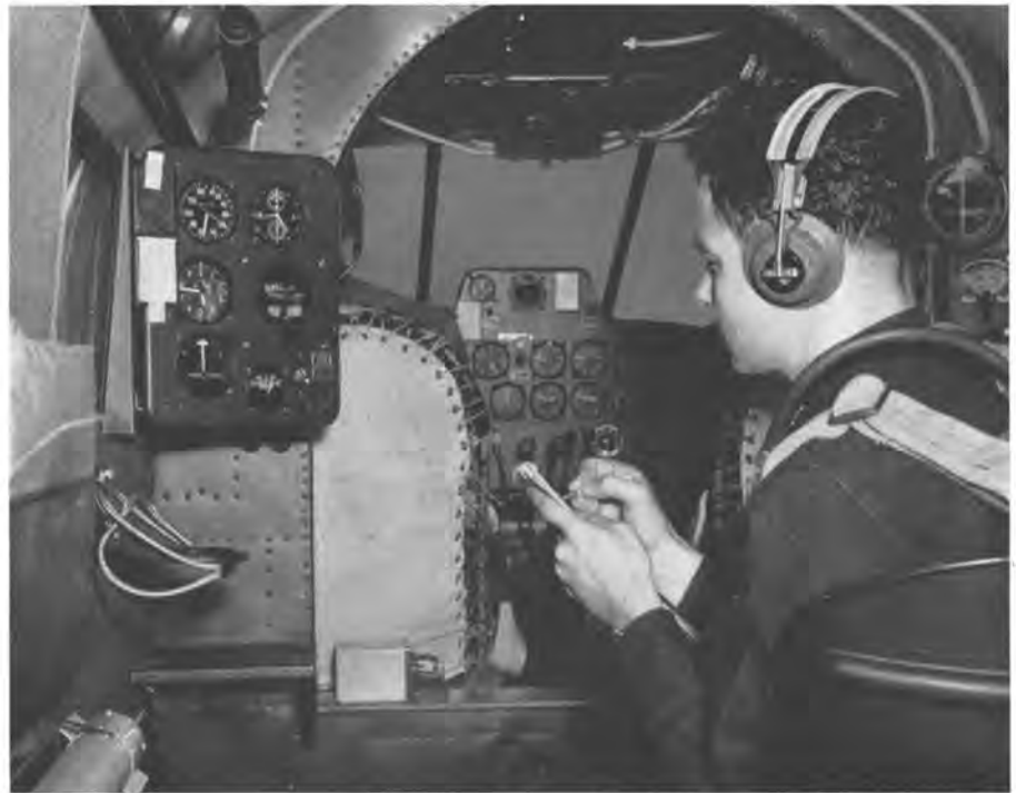
Official Photograph, U.S. Army Air Forces Important equipment within a plane is “interphone,” the telephone system by which all members of the crew may be contacted by the pilot. Here, the navigator of a Beechcraft is “hooked up” with his pilot by interphone, as he takes readings from dials at left
