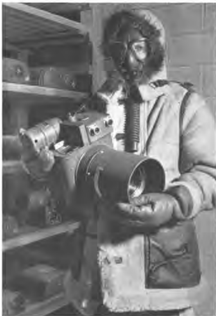
This aerial camera, made by Kodak for the Army, soon will be photographing enemy territory from altitudes of 40,000 feet and more. Here, in the Arctic Chamber at Camera Works, it is about to undergo low-temperature tests more severe than any it will meet in actual use. Other climates are also offered by the weather-wise Camera Works
