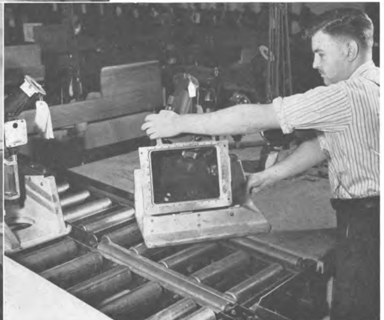
From top left, clockwise: Joseph Ambros places a Navy telescope in cradle that will bear it over rollers on its trip down a Hawk-Eye conveyor line. Albert DeGraff guides instrument onto workbench. George Reimuth removes a telescope from the conveyor line for inspection. Franklin D. Leffler sights a telescope on a distant target to check its precision and cleanliness. Note, incidentally, Kodak Park's twin chimneys visible through window. At left is a general view of the conveyor line with (left background) Joseph Wardynski and Astrid Coene, and (at right) Mary Ann Vallone, Helen Stremick, Lucille Peters, and Dorothy Linkner working on the Navy telescopes. Hawk-Eye's use of assembly-line technique in the production of these high-precision instruments has increased output without lowering quality
