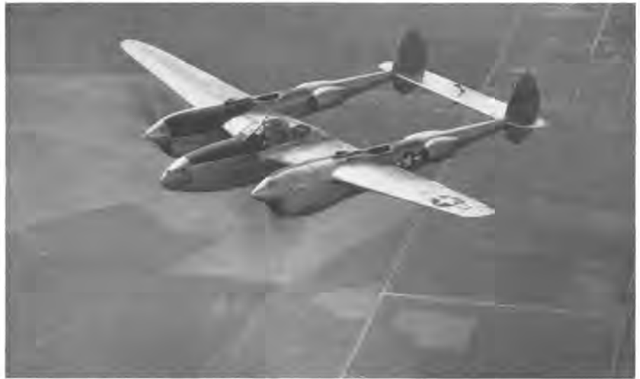
Official Photograph U.S. Army Air Forces Stripped of its guns, the speedy Lockheed Lightning P-38, long-range pursuit plane of the U.S. Army Air Forces, has become one of the "eyes" of the Army in a new role as the F-5 reconnaissance plane. Strictly an unarmed aircraft, sole function of the F-5 is making successful combat possible by performance of its job of aerial photographic mapping. The guns and firing mechanism of the P-38 were removed to make room for the camera and photographic equipment (see lower picture). Cameras are adjustable for most conditions by remote control from the cockpit
