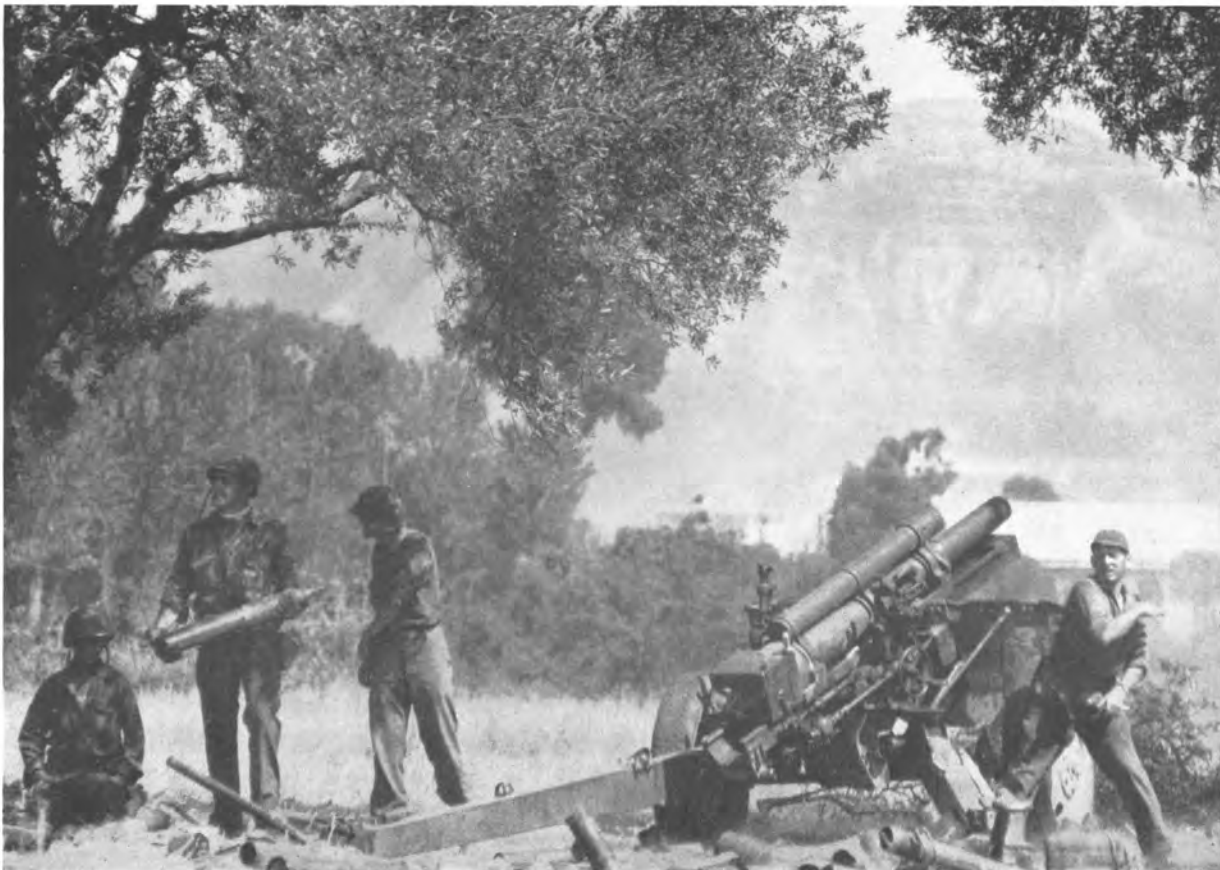
Somewhere on the hard-fought Italian front a U.S. sergeant yanks the cord of a 105-mm. howitzer to blast an enemy position. The telescope used on this gun is the M-12, which is made in large numbers by Kodak
