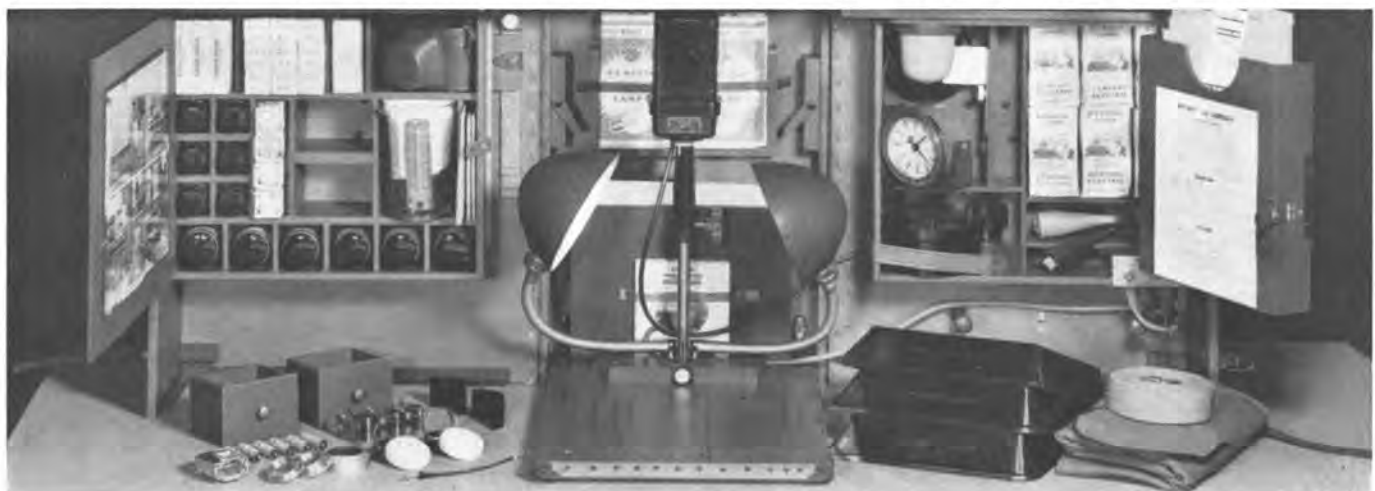
Here, the handy compartments, shelves, and drawers of the laboratory in a suitcase are shown. Equipment for taking pictures includes a Kodak 35
