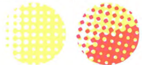
Magnified 15 times, a print from a section of the "yellow" plate is seen to be a pattern of dots . . .
