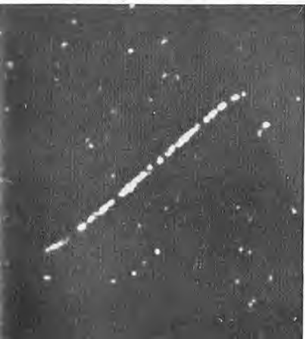
White streak on special photo-plate shows track of uranium atom which was split by a bombarding neutron.
