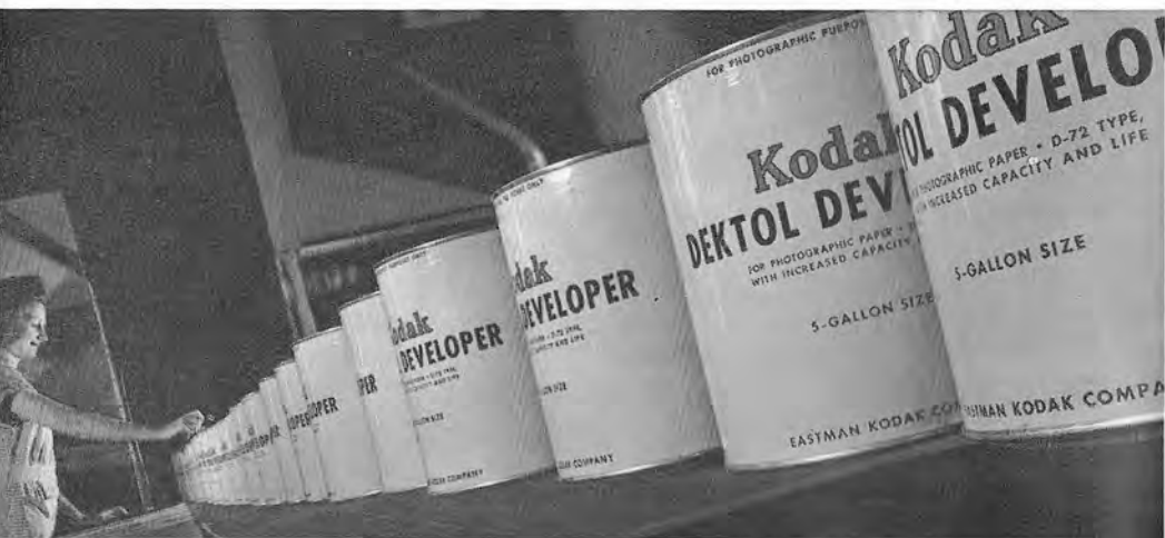
Photographic paper base (above) in storerooms for aging; chemicals (below) being funneled into cans; amateur roll film (opposite page) coming from automatic boxing machine.
