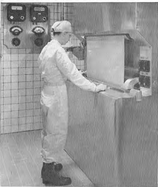
Film base receiving a coating of emulsion.
