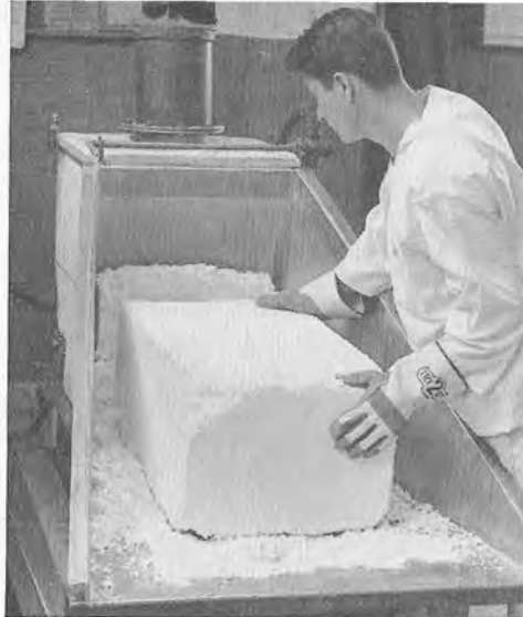
Bale of cellulose acetate being broken up and dumped into a solution containing solvents.
