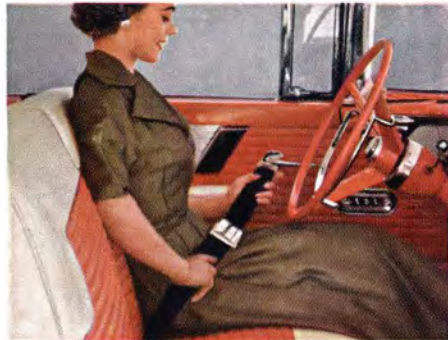
8. New safety seat belts* —bolted to floor supports—are available for driver and passengers. Made of durable high-strength nylon, they are designed for easy one-hand adjustment.
