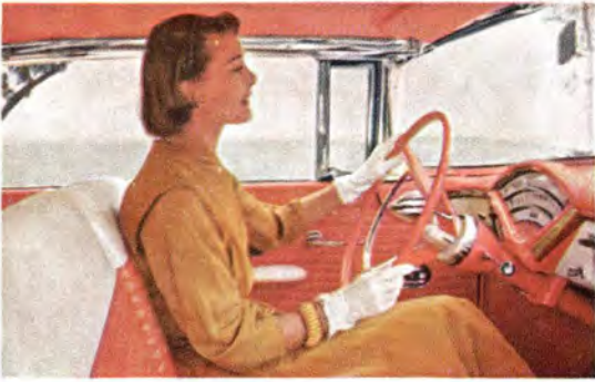
1. New impact-absorbing safety steering wheel , with deeply recessed hub, offers greater protection for the driver during quick stops. The wheel is also positioned for better visibility.
