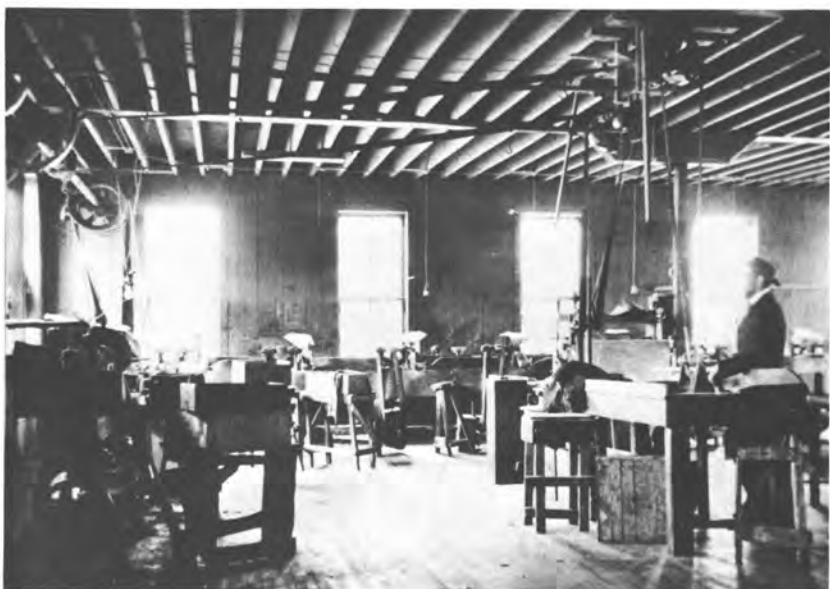
Interior of pipe factory, Mumford, N.Y. Harry Harvey in picture with machines used to buff and polish pipes made of applewood.
