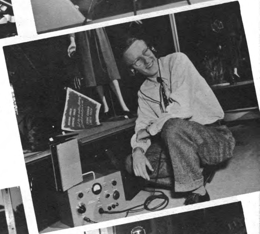
Right: Bob Treacy takes a field-strength reading in downtown Rochester.
